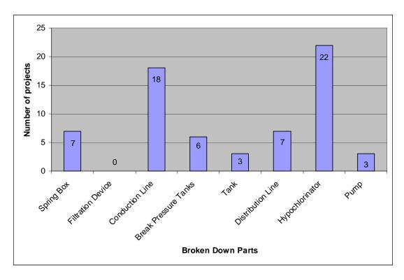
**Comment:** As indicated earlier, in 22 of the 32 visited communities, there are problems with hypo-chlorinators although 68% of these problems were fixed in less than 3 days. Importantly, problems with the conduction line (i.e. transmission line) are also regular (18 of 32), although this is to be expected since pipes were regularly laid unprotected in drainage ditches, which allows them to be washed away during storms. This issue needs to be addressed in the future.
